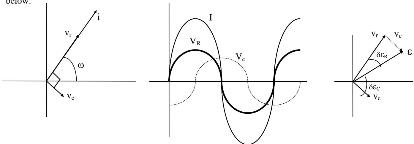
Because of the combination of the resistor and the capacitor in the circuit, a phasor vector  $\epsilon$ , as shown in the third figure from left above, can represent the voltage across the entire circuit. Note that this vector is equal to the sum of the two sine waves for the voltage across the capacitor and the voltage across the resistor.
