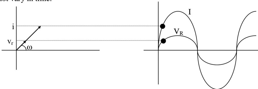
So, the current at that moment in time ( $i$ ) is the vertical component of the  $I$  vector which rotates with an angular frequency  $\omega$ . The voltage across the resistor ( $v_r$ ) at that moment is the vertical component of the  $V_R$  vector that rotates with an angular frequency  $\omega$ .
